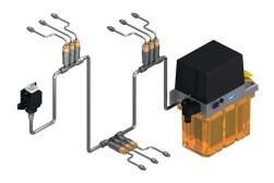
Mainly intended for use in small and medium-sized machines, the **SKF MonoFlex Standard** single-line system carries oil, fluid grease and other grease. With every lubrication impulse, 0.01 to 2.5 cm³ of lubricant is conveyed to all connected lubrication points. A piston metering valve on each lubrication point ensures precise dispensation, regardless of viscosity and counterpressure.
