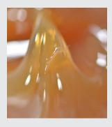
Klüberplex HB 98-601 sample after testing at more than 200 °C for 3 hours
